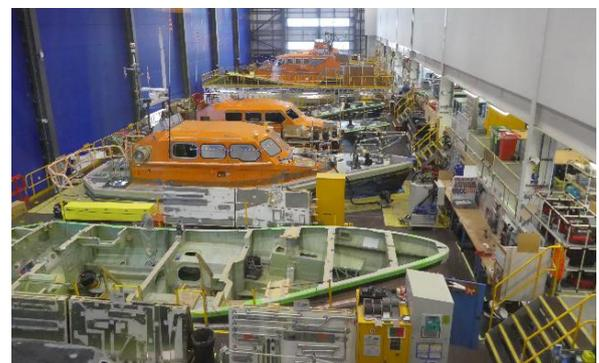
together and transferred to the paint shop then returning for second stage fitting out including the systems and information management systems, communications, navigation and machinery monitoring. There are six production stages in total each of 8 weeks. The factory has a component manufacturing section and areas for recovery and storage of the lifeboats.
