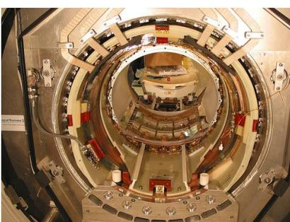
X-rays coming from an X-ray tube to one side are measured by the detectors on the other side of the patient. The amount of absorption of the X-rays as it passed through the body being the difference between the readings at each detector and the reference detector that has nothing in its path. The readings are converted into a digital number and stored in the computer.
