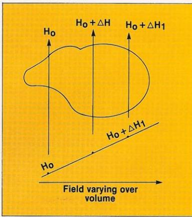
Some additional coils, namely the gradient coils, apply a small gradient to the value of the field in a particular direction is made to vary linearly along that line. It is a small variation compared to the strength of the main field but enough to make a difference to the frequency of resonance of the protons.
